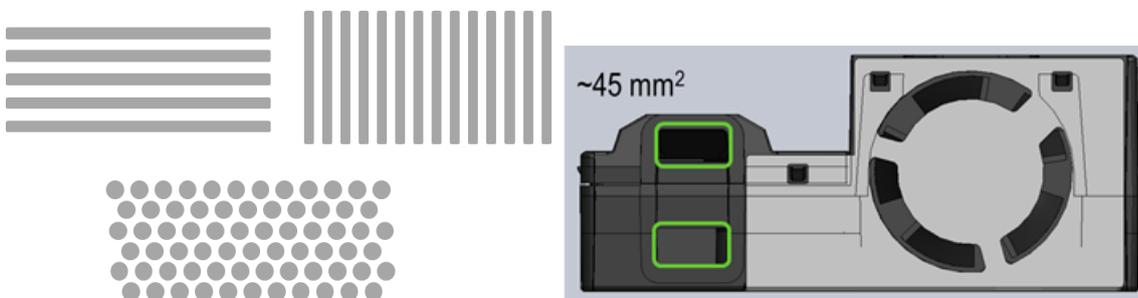
An important requirement is that the openings in the housing do not restrict the air flow through the sensor.
