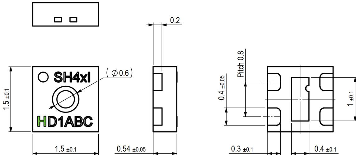
**Figure 2.** Dimensional drawing of SHT4x including package tolerances (units mm).
