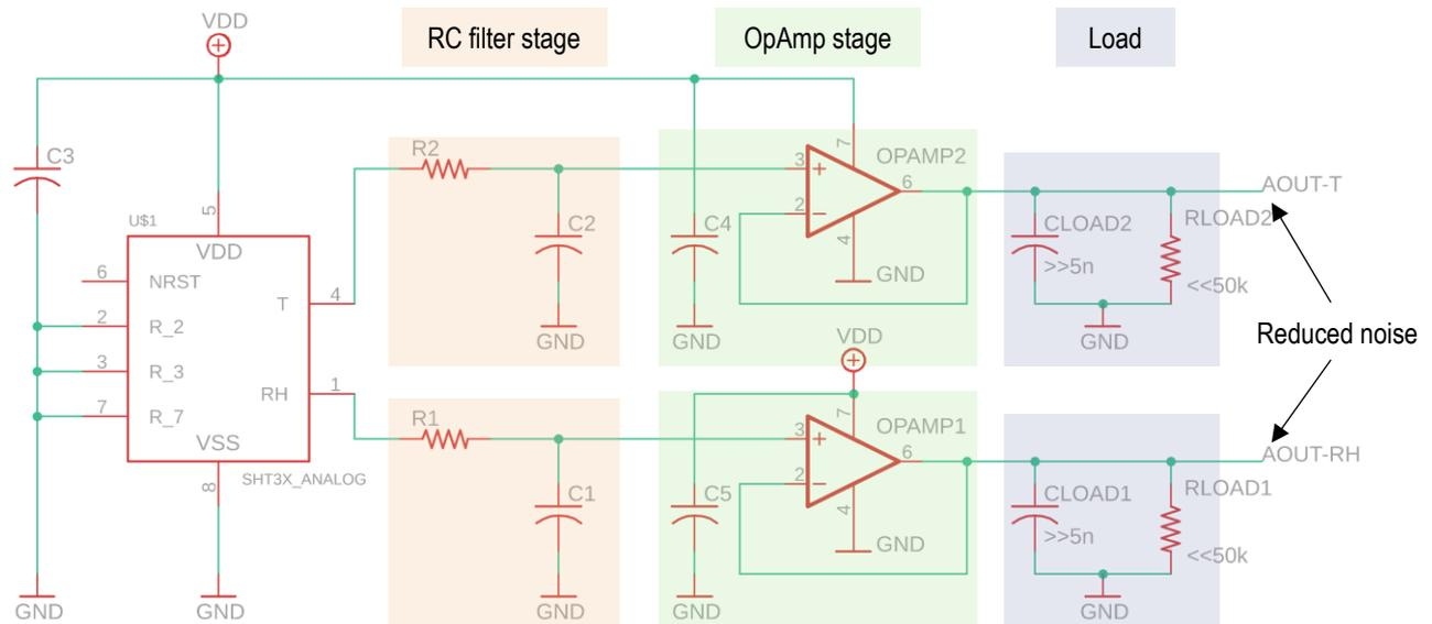
**Figure 4.** Possible improved schematic for the SHT3x. This solution allows greater drive capability and reduces output noise. However, it considerably increases the overall costs of the final product.
