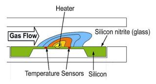
The mass flow sensing element is integrated on a CMOSens® chip allowing the signal to be amplified and digitized on chip for best performance.
