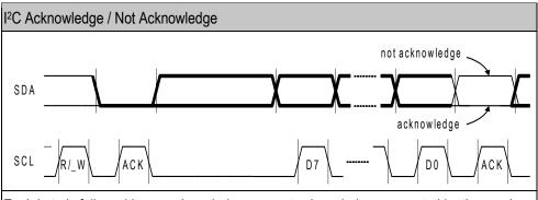
Each byte is followed by an acknowledge or a not acknowledge, generated by the receiver (The bold lines indicate that the sensor controls the SDA line)
