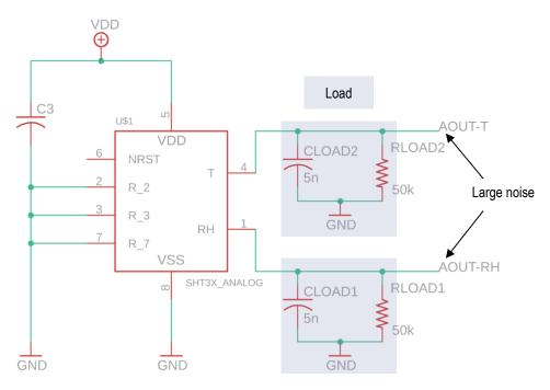
Figure 3. Standard schematic for the SHT3x. Load is directly connected to the sensor, but there is large noise at the output.
