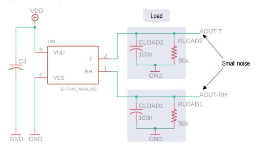
Figure 5. Standard schematic for the new SHT4xI analog sensor. Significant loads can be directly connected to the sensor and the output signals have negligible noise.
