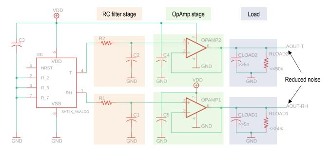
**Figure 4.** Possible improved schematic for the SHT3x. This solution allows greater drive capability and reduces output noise. However, it considerably increases the overall costs of the final product.
