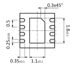
Figure 1. Dimensional drawing of the SHT3x including (units mm).
