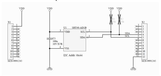
Figure 1: Schematic Diagram of the SENSEVAL-SHT4XV1
