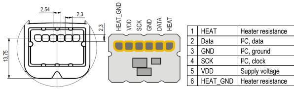
Figure 4. PCB pad layout of sensor
