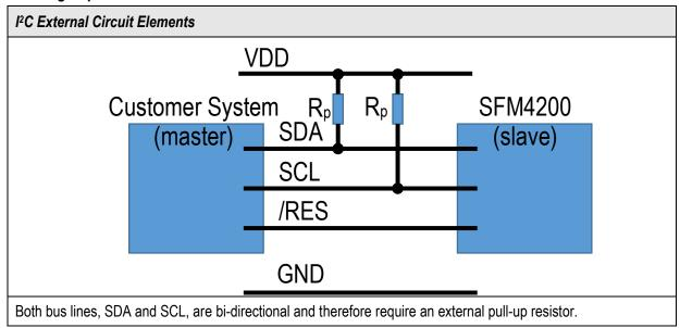
Communication between a master and the SF05 sensor system runs via the digital I<sup>2</sup>C-interface. For detailed specifications of the I<sup>2</sup>C protocol, please refer to the document "The I<sup>2</sup>C-Bus Specification, Version 2.1, January 2000" from NXP (http://www.nxp.com/products/interface\_control/i2c).
