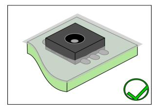
Instruction 5. If conformal coating is applied, the top surface of the sensor must remain free of coating.
