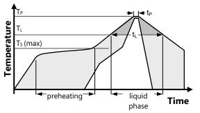
**Figure 1.** Soldering profile according to JEDEC standard.  $T_P \le 260$  °C and  $t_P \le 30$  sec above 255 °C for Pb-free assembly.  $T_L < 220$  °C and  $t_L < 150$  sec. Ramp-up rate <3 °C and ramp-down rate <6 °C/sec for temperatures > $T_L$ .
