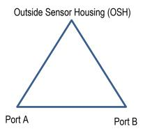
In this triangle, the differential pressure on any leg (i.e., A-OSH, B-OSH, A-B) must not exceed the overpressure or burst pressure defined in the product datasheet.
