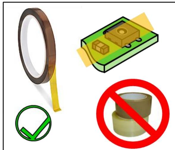
**Instruction 7.** In conjunction with the sensor, use only recommended Kapton® tape Electrical Tape 92 by 3M™. Do not apply any other adhesive tapes such as Scotch Tape, Sello Tape, Tesa Film etc.
