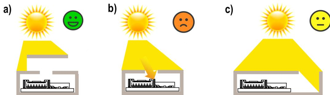
**Figure 4:** Sensor protection from sunlight (connector view). **(a)** Good protection and **(b)** bad protection from incoming sunlight. **(c)** Good protection from sunlight, however, at the cost of bad coupling to ambient and a large dead volume.
