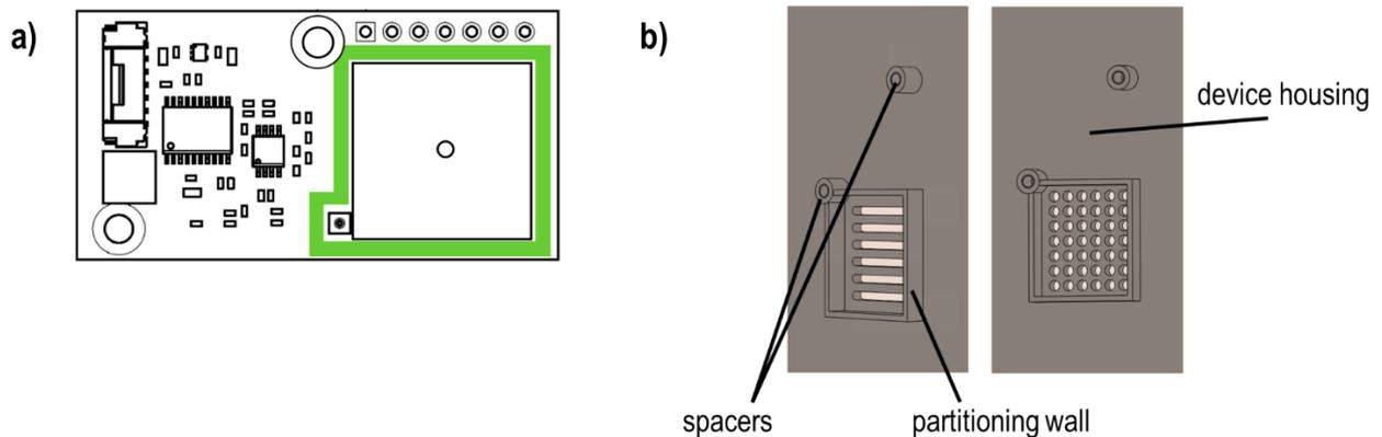
**Figure 7:** Sealing and shielding around the sensing elements of the SFA30 sensor module to prevent or at least reduce the impact from local environmental conditions inside the device on the sensing performance **(a)** Top view: area marked in light green to be used for sealing or shielding purposes and **(b)** Internal view of device housing: exemplary implementation of partitioning walls surrounding the sensing elements including two possible aperture designs.
