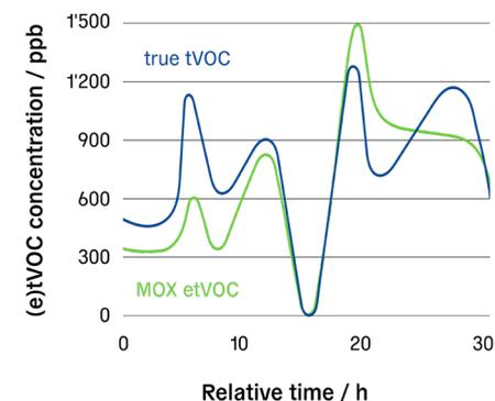
The plot above shows a typical field situation for VOCs. Due to its nature, the etVOC output of a typical MOX sensor deviates significantly from the true tVOC concentration. Some events may even not be detected by the MOX sensor if it is not sensitive enough to this particular VOC.
