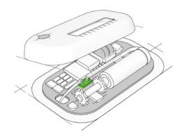
In contrast to pump actuation, a flow sensor provides a direct flow measurement, enabling real-time tracking of administered doses and rates. Integration of drug temperature and media detection are additional ways to ensure compliance.
