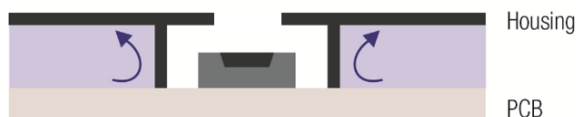
Figure 2: Sealing of the sensor compartment towards the remaining housing minimizes the influence of entrapped air on the sensor.
