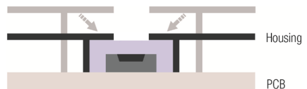
Figure 3: A small dead volume allows for rapid adaption to changes in the environment.
