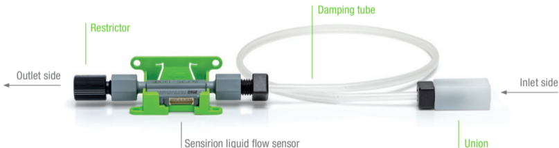
Components of Sensirion's pulsation damping kit (labeled in green); example setup with the SLF3S-1300F
