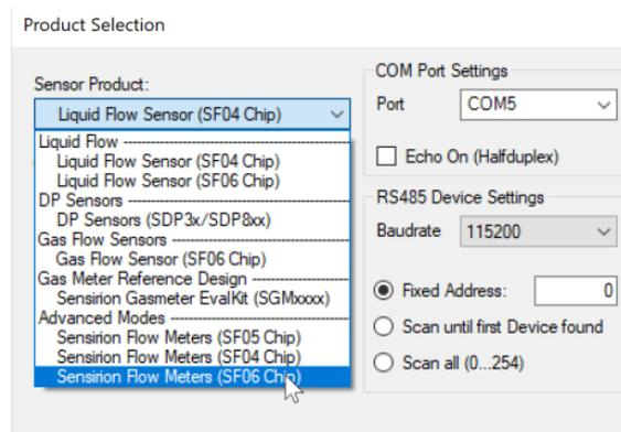
Afterwards the sensor viewer starts in advanced mode in which the generated HEX-command can be entered in the box in the left part. Please not that in advanced mode, the scale factors and units of the sensor must be entered manually.
