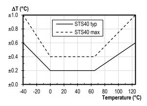
Figure 2. STS40 typical and maximal temperature accuracy.
