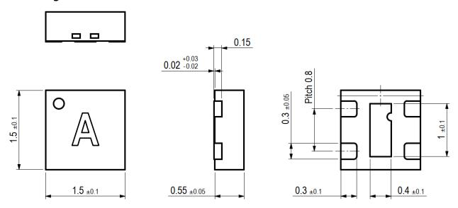
**Figure 4.** Dimensional drawing of the STS4x including package tolerances (units mm). The Pin 1 is identified by the laser dot on the top side and the cutout of the die pad, visible from the bottom. In the middle of the DFN top side, a lasered character ("A", "B", or "C") indicates the I2C address as detailed in **Tables 7 and 8**.
