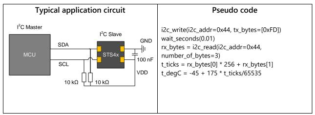
Figure 1. Typical application circuit (left) and pseudo code (right) for easy startup.
