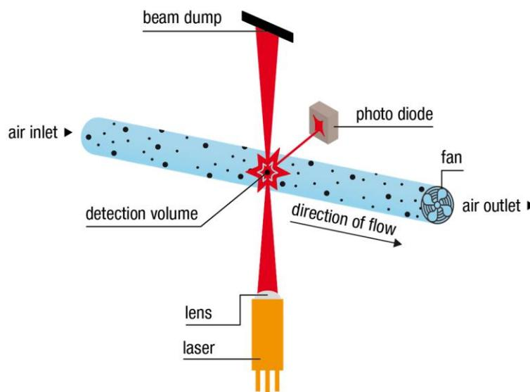
**Figure 1** Measurement principle of Sensirion PM sensors.
