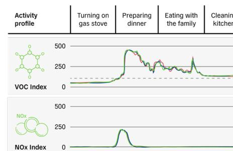
The figure at the top demonstrates a possible example implementation of the NO<sub>x</sub> Index in an air purifier. At the bottom, one can see a typical activity profile in a kitchen for which the simultaneous monitoring of VOC and NO<sub>x</sub> Indices helps distinguishing different types of events.
