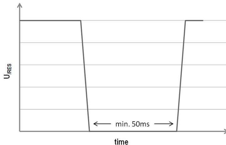
To ensure that the power to the SF05 flow chip is correctly interrupted during the reset, also pull down the SDA and SCL lines at the same time as pulling down the /RES line.
