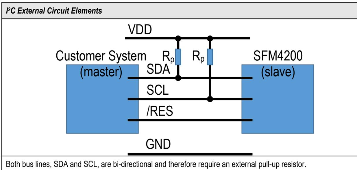
Communication between a master and the SF05 sensor system runs via the digital I<sup>2</sup>C-interface. For detailed specifications of the I<sup>2</sup>C protocol, please refer to the document "The I<sup>2</sup>C-Bus Specification, Version 2.1, January 2000" from NXP ([http://www.nxp.com/products/interface\\_control/i2c](http://www.nxp.com/products/interface_control/i2c)).
