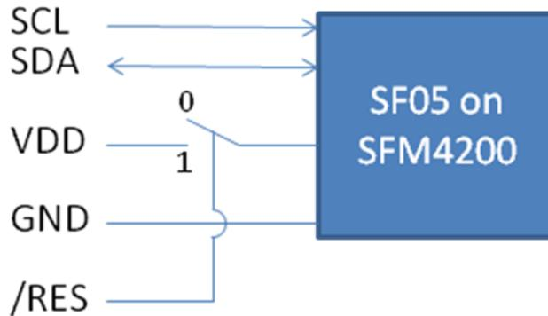
Input equivalent circuit:
