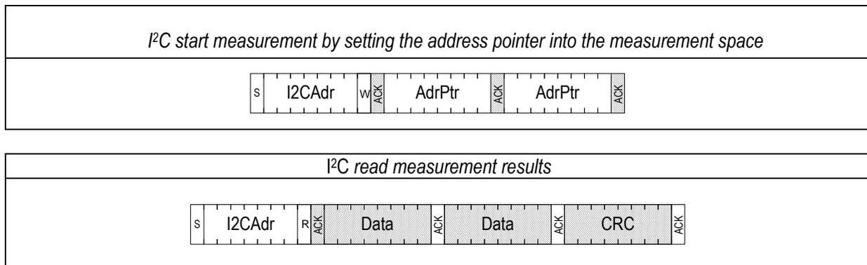
The CRC byte is calculated using the generator polynomial  $G(x) = x^8 + x^5 + x^4 + 1$  (hex 0x31). The initial value is 0.
