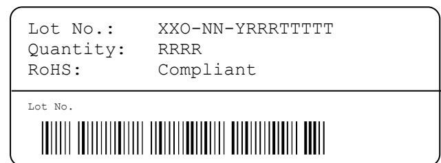
Figure 12: First label on reel: XX = Sensor Type (20 for SHT20), O = Output mode (D = Digital, P = PWM, S = SDM), NN = product revision no., Y = last digit of year, RRR = number of sensors on reel divided by 10 (200 for 2000 units), TTTT = Traceability Code.
