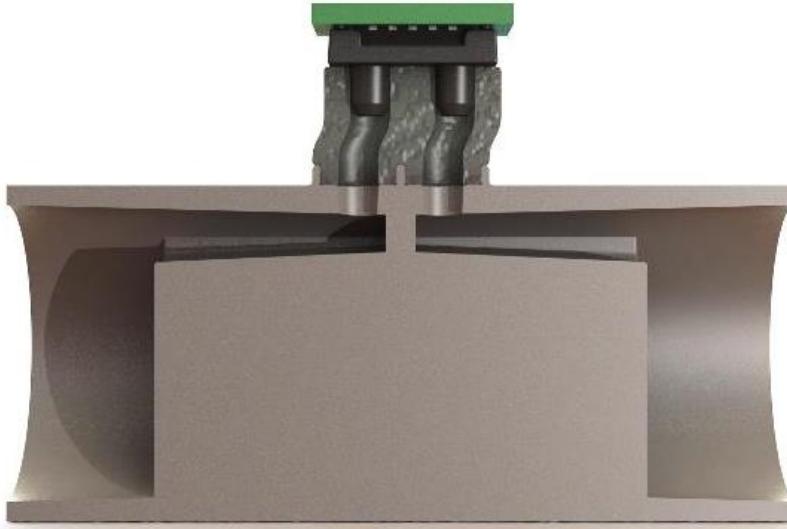
Figure 5.3: Soft adaptor between flow channel and manifold
