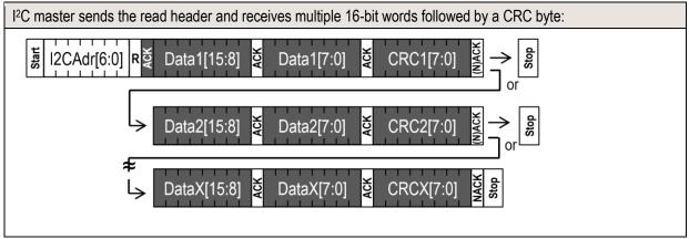
Figure 3: I<sup>2</sup>C sequences to read results from the sensor. Dark areas with white text indicate that the sensor controls the SDA (Data) line. I<sup>2</sup>C sequences can be aborted with a NACK and STOP condition.
