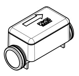
Tolerance on O-ring diameter: (16.6+/-0.08)mm
