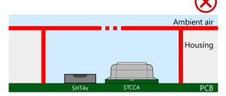
Guideline 1: Design a sufficiently large aperture to ambient air.
