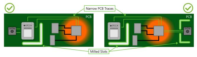
**Guideline 1**: Maximize the distance between the sensor and heat-generating components. **Guideline 2**: Use milled slots and narrow PCB traces to minimize heat conduction through the PCB.
