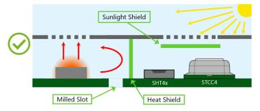
**Guideline 3**: Shield the sensor with heat shields or pockets from heated air. **Guideline 4**: Protect the sensor from direct sunlight exposure.
