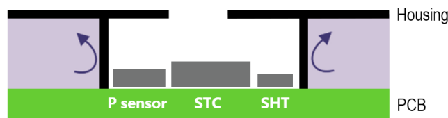
Figure 5. Pocket sealed from device's inside
