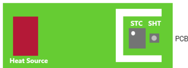
Figure 2. Decoupling the sensors from heat sources by adding slits or holes in the PCB design
