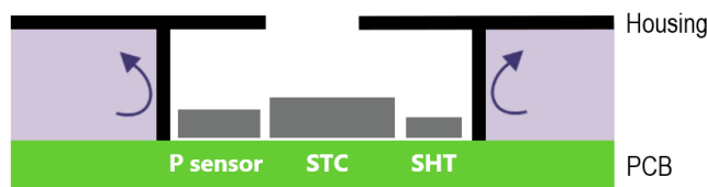
Figure 5. Pocket sealed from device's inside
