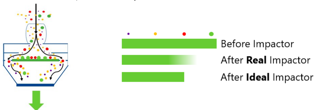
Figure 2. Gravimetric sensing: gradual separation rather than binary in impactor.
