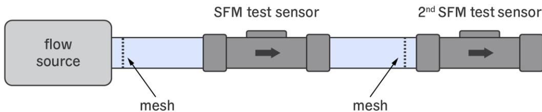
Figure 2. Recommended Initial Test Setup with SFM Modules
