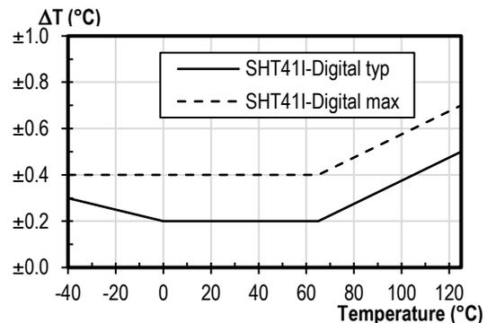
**Figure 5:** SHT41I-Digital typical and maximal temperature accuracy.
