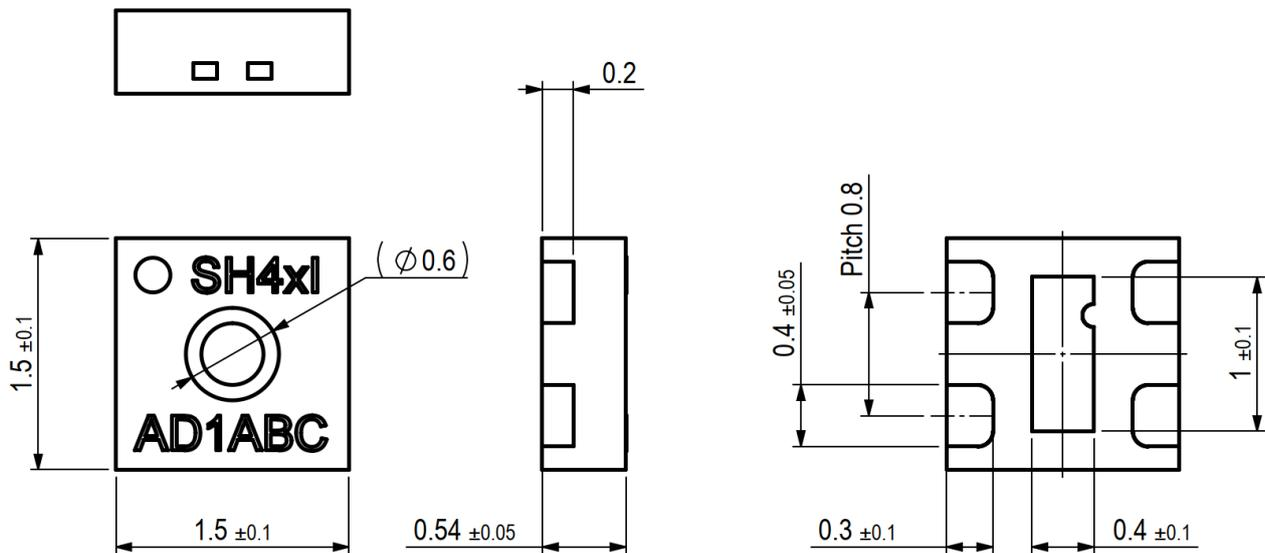
**Figure 7** Dimensional drawing of SHT4xl-Digital including package tolerances (units mm).
