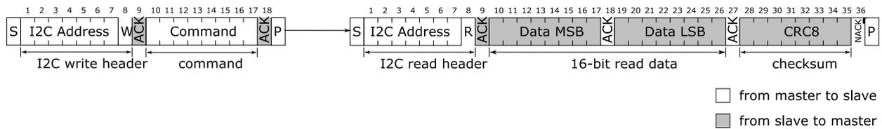
**Figure 6:** I2C transfer types: First a write header is sent to the I2C slave, followed by a command, for example “measure RH&T with highest precision”. After the measurement is finished the read request directed to this I2C slave will be acknowledged and transmission of data will be started by the slave (here, only the temperature values are transmitted for reasons of simplicity).
