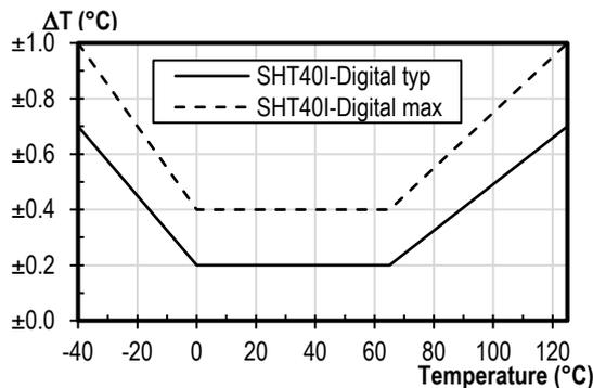
**Figure 4:** SHT40I-Digital typical and maximal temperature accuracy.
