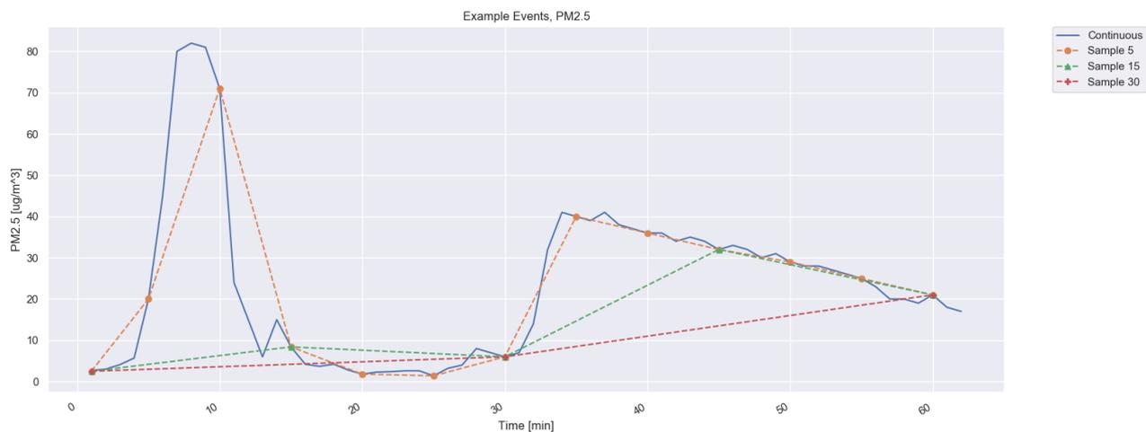
Figure 6: Example of fast event and slow event with different sampling time intervals
