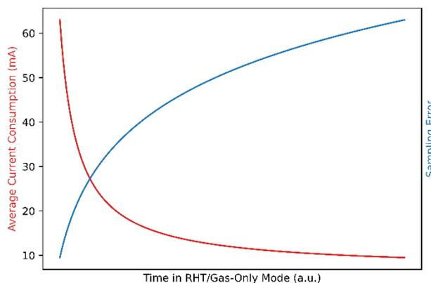
Figure 3: Schematic drawing showing the interplay between reducing average current consumption and increasing the sampling error. It is assumed that the sensor is cycled between the full Measurement Mode for fixed time and then switched to RHT/Gas-only Measurement Mode for x time, where x is plotted on the horizontal axis. Time is in arbitrary units (a.u.) since quantitative estimates depend strongly on the type and dynamics of particle events.
