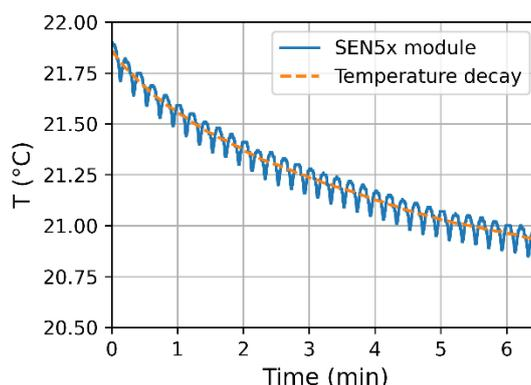
Figure 4: Automatic compensation of SEN5x. The orange dashed lines shows the overall (averaged) temperature trend, the blue line shows the temperature measured by the SEN5x module while switching between gas only and full measurement mode. Offsets and saw-tooth behavior in the compensated and uncompensated T-signals can be observed, depending on the design-in and cycle's parameters.
