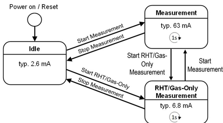
Figure 1: The different operating modes of the SEN5x sensor.
