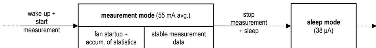
Figure 2: Illustration of one complete cycle of low-power operation. The first phase in measurement mode is characterized by the fan starting up and the PM algorithm accumulating statistics. During this phase the measurement data of the SPS30 is not stable and shall not be used.
