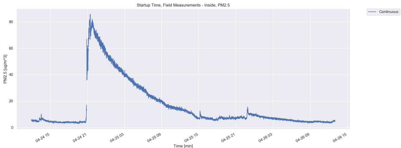
Figure 4: A typical indoor cooking event with fast increase and a slow decrease, measured in continuous measurement mode.
