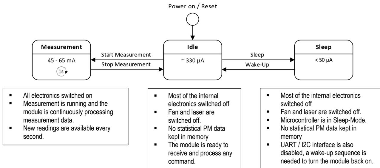
Figure 1: The different operating modes of the SPS30 PM sensor.
