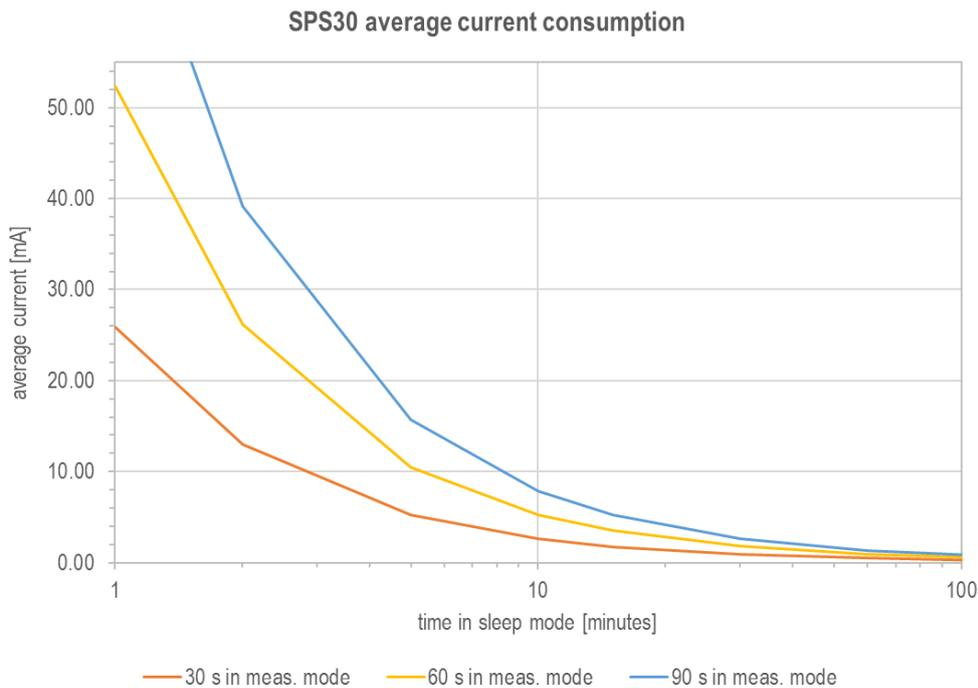
Figure 7: Average current consumption for different times in measurement (30/60/90 seconds) mode and sleep mode (from 1 minute to 100 minutes). Please note the logarithmic scale of the x-axis.
