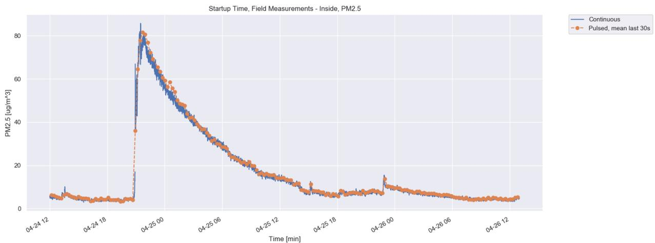
Figure 6: A typical indoor cooking event with fast increase and a slow decrease can be perfectly measured with the proposed implementation example. Blue curve: continuous measurement. Orange curve: 60 seconds measurement time represented by one data point as an average of the last 30 seconds, 15 minutes sleep time.
