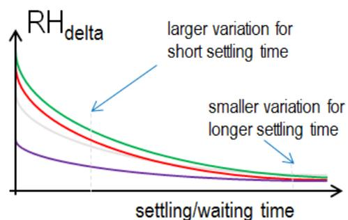
Figure 13 Graph showing  $RH_{\text{delta}}$  measurements of several units over time. The longer the waiting time the more accurate is the measurement (the closer it is to the final value).
