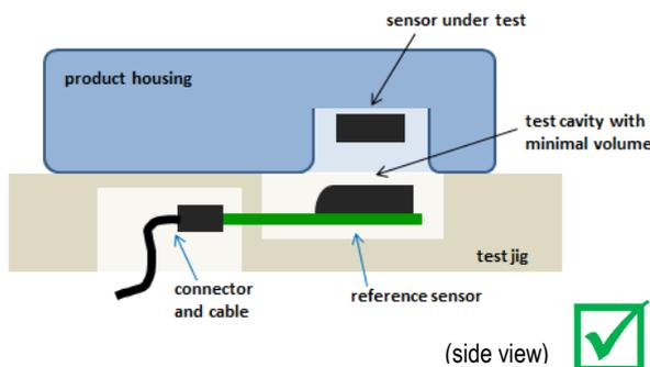
Figure 9 Good example of test jig for sensor in a housing, with sensor under test aligned just next to the reference
