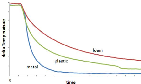
Figure 2 Exemplary data showing several sensors approaching reference value. Different materials have been used to couple the sensors to the reference sensor. Metal offers the best thermal coupling, resulting in the fastest settling times. Coupling sensors through e.g. plastic or foam requires significantly longer settling times and may lead to less accurate measurements.
