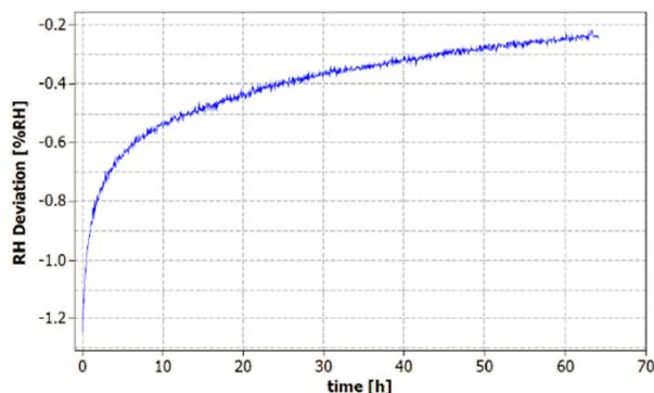
Figure 17 Mean deviation from initial calibration when sensor is exposed to ambient conditions of 25°C and 50 %RH directly after reflow soldering process (representative plot)
