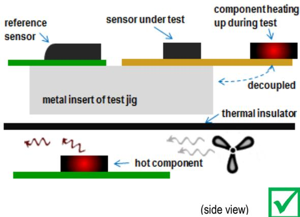
Figure 5 Good example of PCB test jig with the metal insert being decoupled from components on the DUT that heat up during test. Metal insert is insulated from the self-heating of the electronics inside the jig. Additionally the electronics of the jig are ventilated to prevent too much self-heating.
