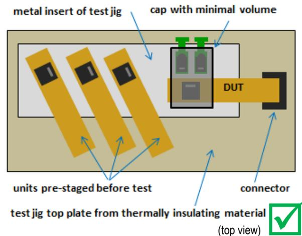
Figure 7 Good example of test jig top plate from thermally insulating material (e.g. plastic), preventing the operator to easily touch the metal insert of the test jig. The metal insert is large enough to provide space for pre-staging several units before test, allowing the units to adjust to the temperature of the jig.
