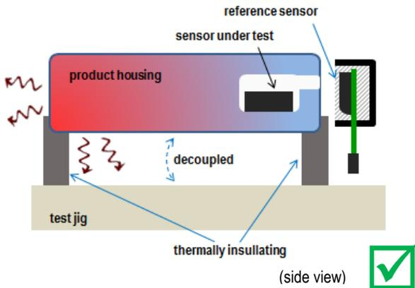
Figure 12 Good example of self-heating unit, placed on thermally insulating stilts to decouple it from the test jig surface, preventing heating up of the jig. Note that the cap around the reference sensor is as well detached from the device under test, to prevent it from heating up (and no longer represent the environment correctly).
