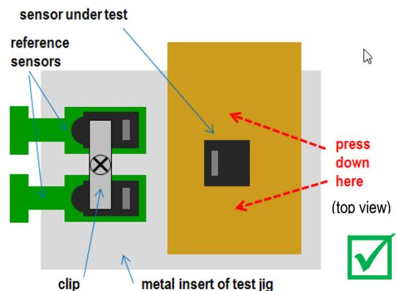
Figure 4 Good example of PCB test jig with clip holding down two reference sensors to ensure good thermal coupling to the metal insert. The reference sensors and the sensor under test are placed at minimum distance to each other.
