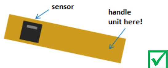
Figure 16 Handle the units before test as far away from the sensor as possible to prevent the operator’s body heat to warm up the DUT.
