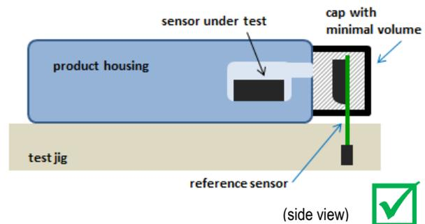
Figure 10 Good example of reference sensor mounted inside a cap, covering the sensor opening of the product housing. The volume inside the cap is minimized, at the same time protecting the sensors from turbulences in the environment.
