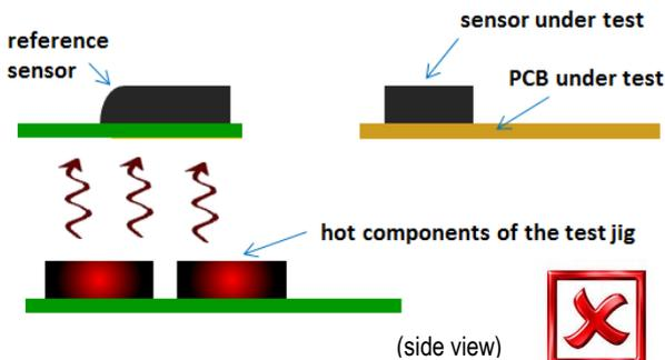
Figure 6 Bad example of PCB test jig. Sensor under test and reference sensor are not sufficiently close together and have to rely on the thermal coupling through air alone. Additionally, there are heat sources below the sensors creating a thermal imbalance.
