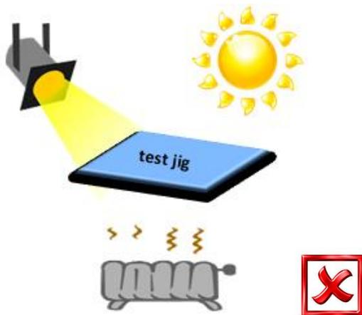
Figure 14 Bad example of a test jig that is exposed to different heat sources – direct sunlight, a strong spotlight and a heating system.
