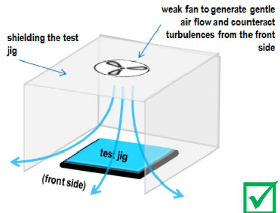
Figure 15 Shielding the test jig to the left/right/back/top reduce turbulences at the test jig. Access for operation is from the front side only. A small fan in the top cover ensures a gentle air flow towards the operator, further reducing the effect of turbulence near the jig.
