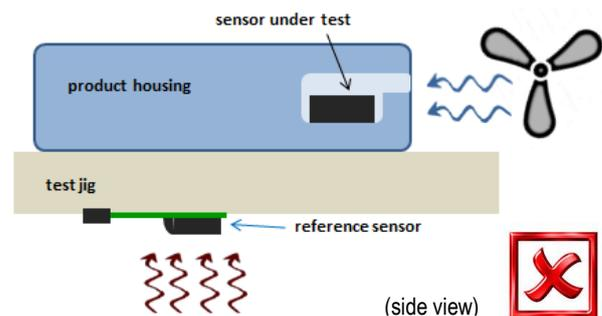
Figure 11 Bad example with reference sensor located far from the sensor under test. Reference sensor is exposed to hot air, while the sensor under test is cooled by a ventilator and/or air conditioning, creating a thermal imbalance. Neither sensor is shielded from turbulences.
