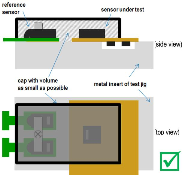
Figure 8 Good Example of small cap enclosing just the reference sensors and the sensor under test, minimizing the volume under the cap as much as possible.
