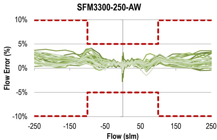
Figure 1. Exemplary flow-error of 30 units SFM3300-250-AW after autoclaving
