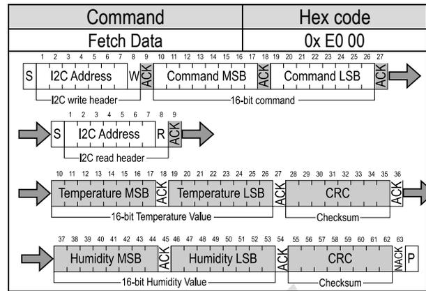
**Table 3.** Fetch Data command (Clear blocks are controlled by the microcontroller, grey blocks by the sensor).
