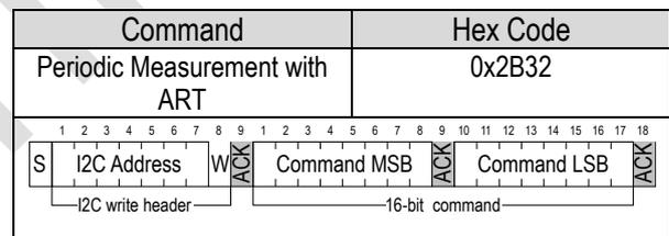
**Table 4.** Command for a periodic data acquisition with the ART feature (Clear blocks are controlled by the microcontroller, grey blocks by the sensor).
