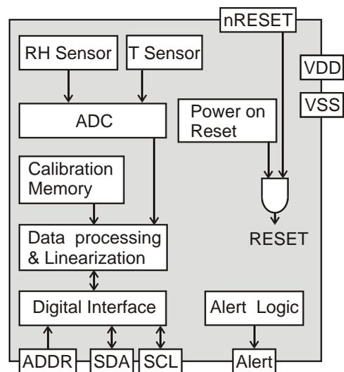
**Figure 1.** Functional block diagram of the SHT33-DIS. The CMOSens™ technology allows providing for a fully calibrated I<sup>2</sup>C signal.
