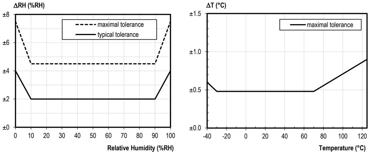
**Figure 2.** Maximal and typical tolerance of  $RH$  at  $25^{\circ}\text{C}$  and maximal tolerance for  $T$ .
