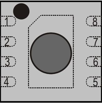
**Table 8.** SHT33-DIS pin assignment (transparent top view). Dashed lines are only visible if viewed from below. The die pad is internally connected to VSS.
