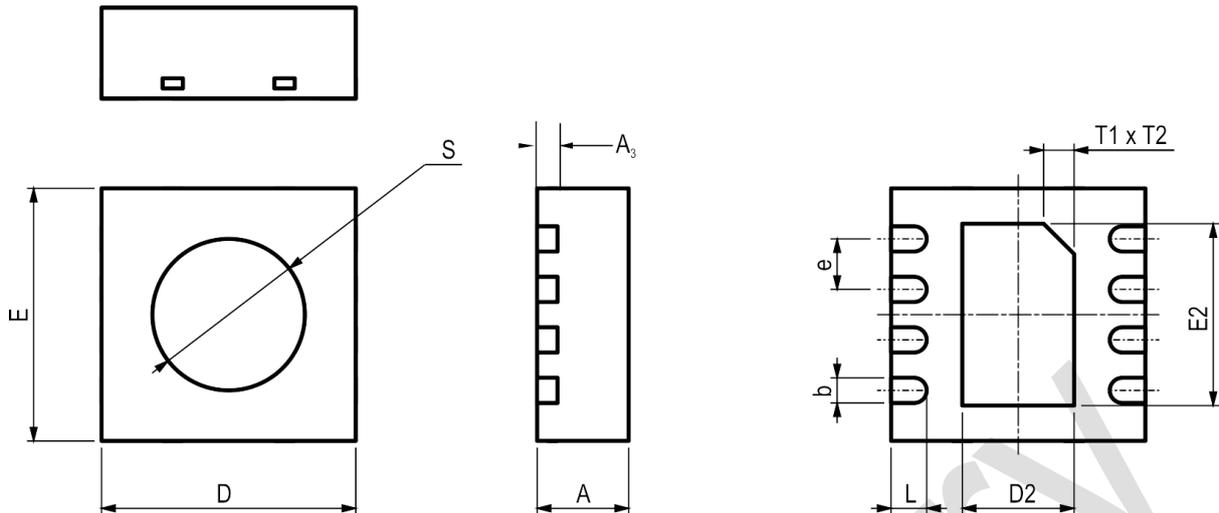
Figure 6. Dimensional drawing of SHT33-DIS sensor package.
