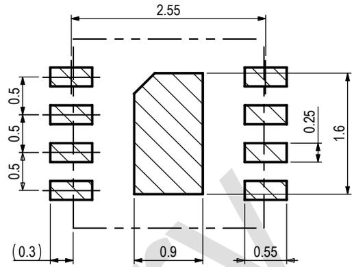
**Figure 7.** Recommended metal land pattern (left) and stencil apertures (right) for SHT33-DIS. The dashed lines represent the outer dimension of the DFN package. The PCB pads (left) and stencil apertures (right) are indicated through the shaded areas.
