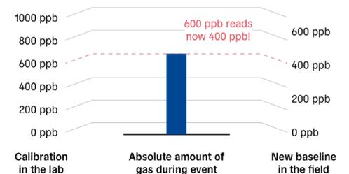
Figures above demonstrate the limitation to provide a concentration output for a specific target gas by a MOX sensor due to broadband sensitivity (top) and varying baseline conditions in the field (bottom).
