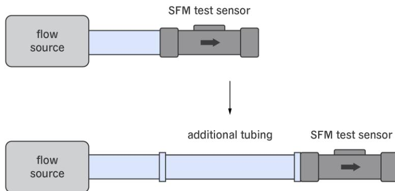
Figure 5. Adding additional tubing or a second reference sensor
