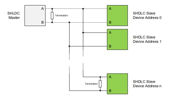
As shown in the picture above, the RS485/422 setup combined with the SHLDC addressing allows to connect several SHDLC devices on the same bus. Due to the differential signals, the communication is robust against disturbances and allows long distance data transmission. For long distance data lines a termination resistor of 120 Ohm is recommended on both ends of the bus. The logic behind the protocol is based on a UART hardware, using the following settings:
