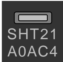
Figure 19 Laser marking on SHT21A. For details see text.
