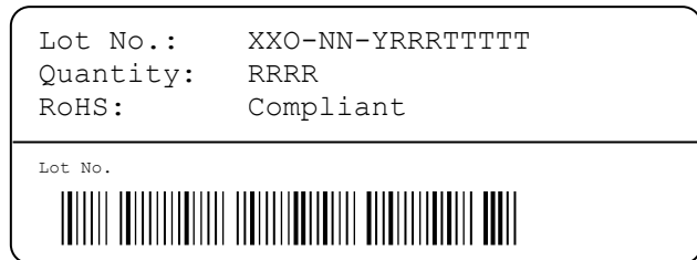
Figure 20: First label on reel: XX = Sensor Type (21 for SHT21), O = Output mode (A = digital, Sensibus and I 2 C, automotive grade), NN = product revision no., Y = last digit of year, RRR = number of sensors on reel divided by 10 (200 for 2000 units), TTTTT = Traceability Code.
