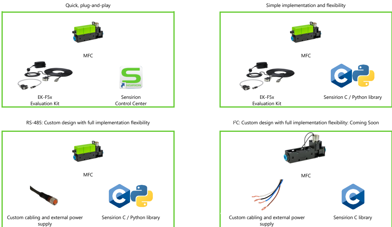
Figure 1. Overview of different options for evaluating digital Mass Flow Controllers and Mass Flow Meters
